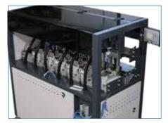
The Automat is used for automatic book-making of up to 8 different washing-care labels from Continuous Rolls of Labels. The automat cuts, optionally folds, collects & puts together 4 to 8 different sizes and lengths of care labels then carries them to the Bartack Sewing head. LB 631 - IX version is equipped with Ultrasonic Cutting system that can cut all various types of label materials in different dimensions.
